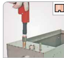
Flat weld Joining two panels
