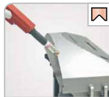
Corner joint Tacking on a cabinet case
