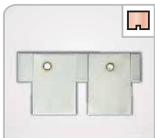
Flat weld Joining panels of different thicknesses
